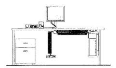
3. Install large-diameter 24" channel horizontally, below desktop. Position small-diameter 17" channel vertically by nearby wall outlet or CPU.
