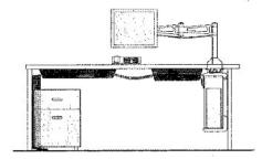
Install large-diameter 17" channel and small-diameter 24" channel horizontally, from end-to-end, below desktop. Position second small-diameter 24" channel vertically, above floor outlet.
