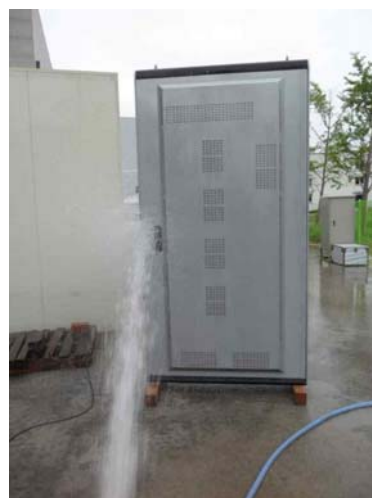
Photo 2. Test for second characteristic numeral 6 with the 12,5 mm nozzle
