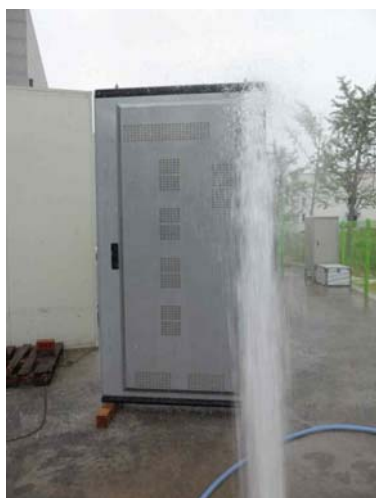
Photo 2. Test for second characteristic numeral 6 with the 12,5 mm nozzle
